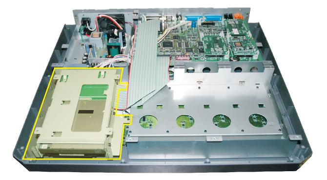
To take out the drive bay remove the four screws as indicated below:
