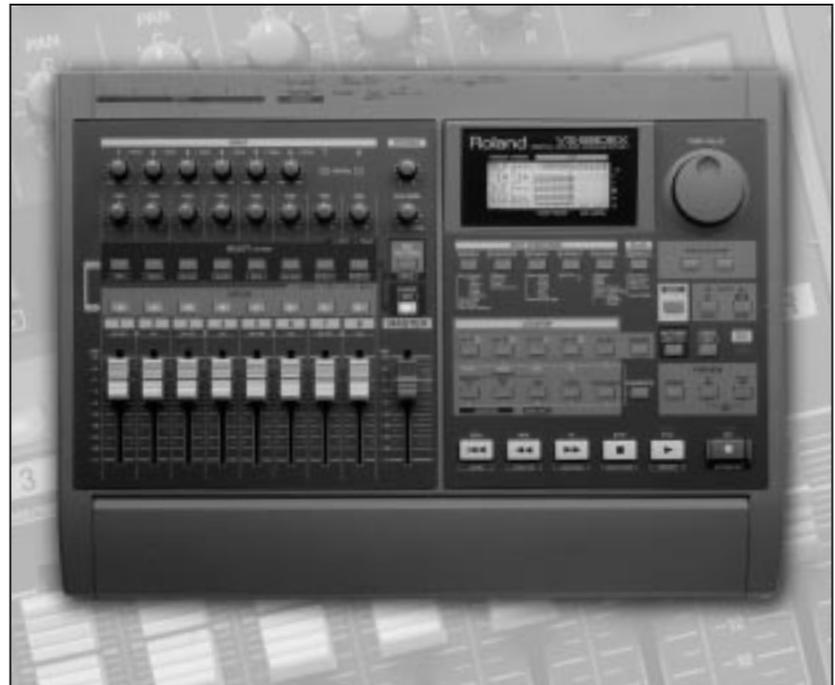
create a new routing simply by holding a Track Status button and pressing any input(s) you want routed to that track. The luminous buttons will flash to confirm the routing you have chosen, greatly speeding up operations.
